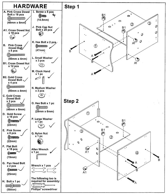
IMPORTANT! DO NOT TIGHTEN SCREWS OR BOLTS UNTIL COMPLETELY ASSEMBLED.
